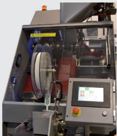
Pantalla táctil con GirControl y etiquetador Wineglass . / Touch panel with GirControl and Wineglass labelling machine.
